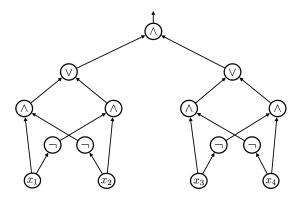
The output gate is the gate at the very top with an arrow that links to nothing. The circuit outputs 1 if and only if  $x_1 \neq x_2$  and  $x_3 \neq x_4$ .
